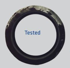
Lip-seal made for Brake Fluid is exposed to Mineral Oil - Pentosin.
